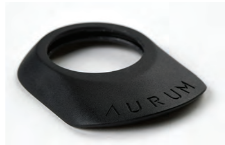
Integrated headset top-cover - made of fiber reinforced composite Available in 8 and 20mm heights Debossed AURUM logo
