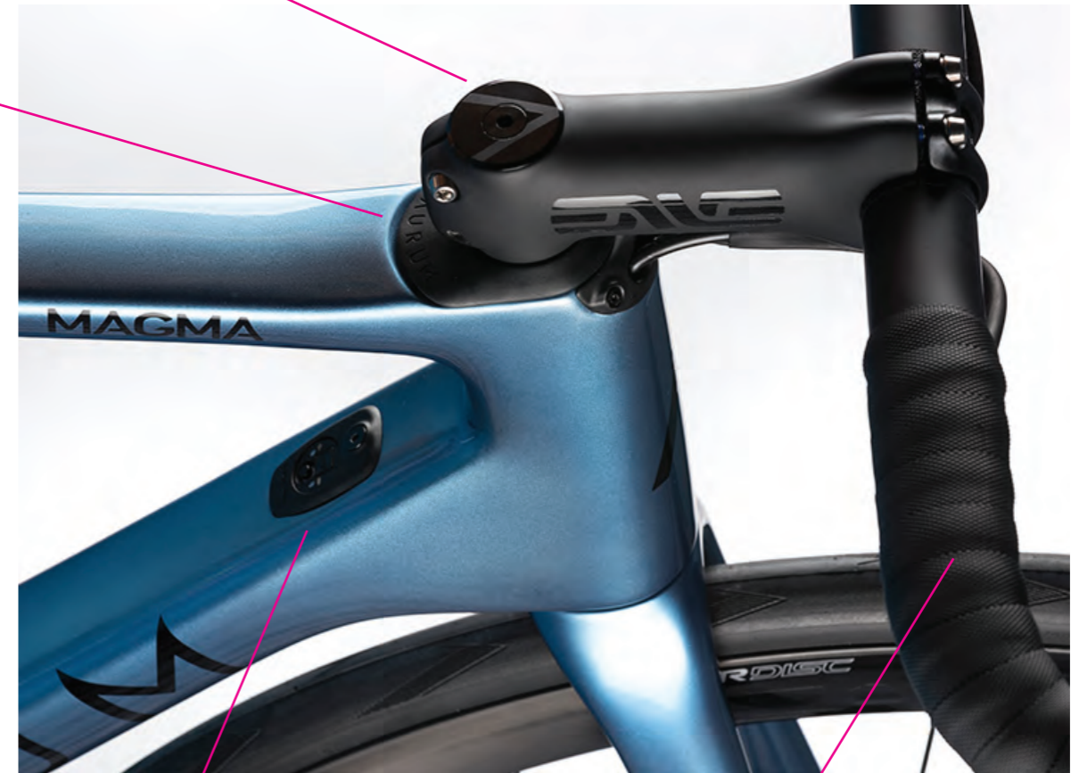
Low-profile, superlight AL-7075 stem top cap and aluminum bolt
